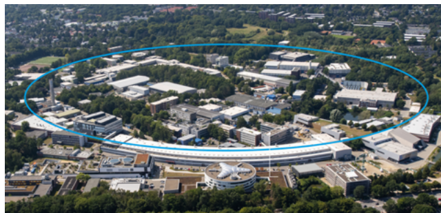
The DESY campus in Hamburg with the 2.3-kilometre-long accelerator ring PETRA III (blue). Three experimental halls – in the foreground the long sweeping arc of the “Max von Laue” experimental hall – and numerous laboratory buildings used by some 20 interdisciplinary scientific institutions are clustered around the ring.
